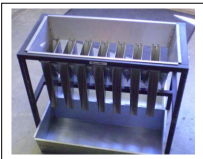
Mechanical Splitter Type B (Riffle)
